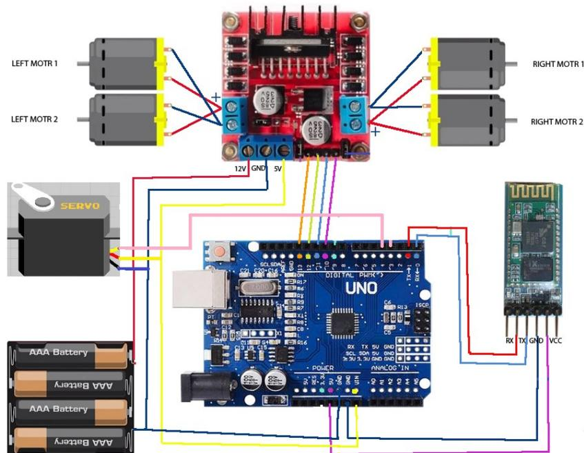
The circuit connections are quite simple, there is one servo motors connected to a pin of the Arduino module that will be used as control inputs for performing arm movements.
