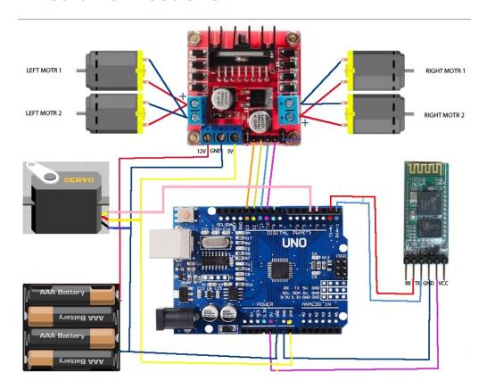
The circuit connections are quite simple, there is one servo motor connected to a pin of the Arduino module that will be used as control inputs for performing arm movements.
