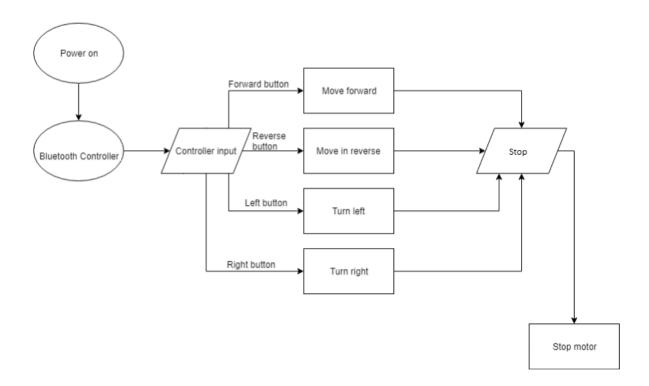
The working of this cricket bot is based on Arduino UNO microcontroller. The block diagram above explains the movement that the car will take in order to reach a specific location on the stage and there are buttons on the app for swinging the bat in a predefined direction. The controller is used for
