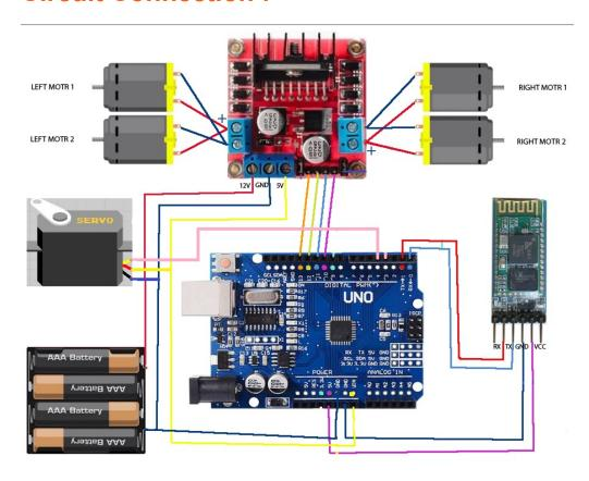
The circuit is quite connections are quite simple, there is one servo motors connected to a pin of the Arduino module that will be used as control inputs for performing arm movements.
